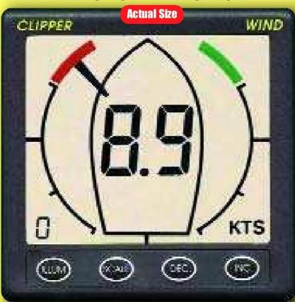
The Clipper WIND showing the speed of 8.9 Knots and wind direction approximately 45 degrees from the port bow
